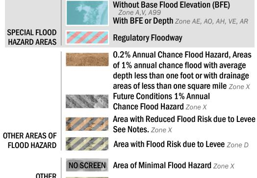
OTHER **Area of Undetermined Flood Hazard** *Zone D* **AREAS** ----- Channel, Culvert, or Storm Sewer **GENERAL** STRUCTURES Levee, Dike, or Floodwall
