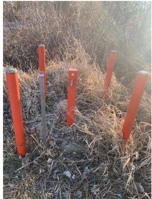
Photo 28: 2020 Typical groundwater monitoring well installed in June 2018.
