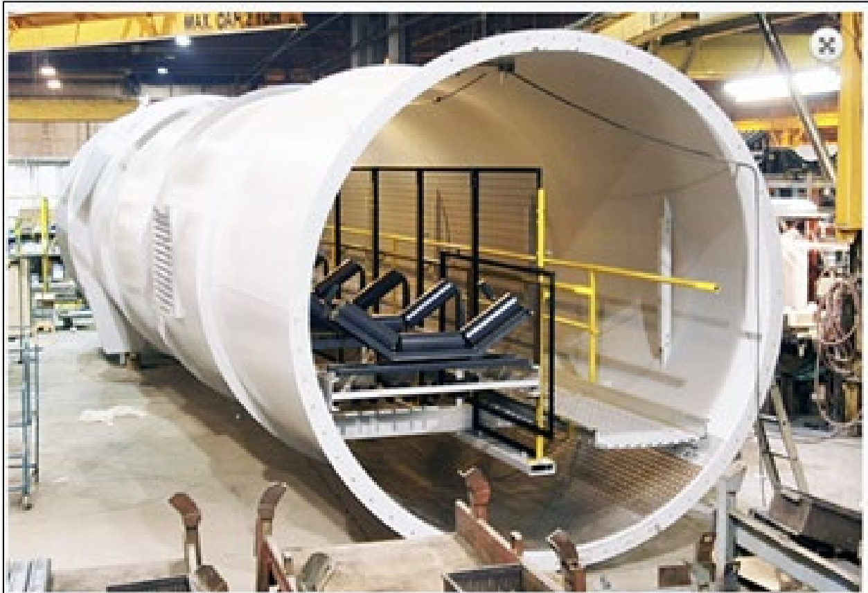
Figure 15: Conveyor Transport System with Tubular Gallery
