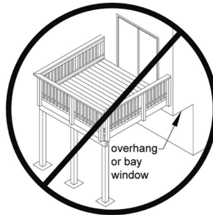
Figure 18. No Attachment to House Overhang with Ledger.
