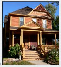
Another excellent Queen Anne example with asymmetrical *facade*, steep roof pitch, and ornamental detailing is seen here. The wrap-around porch to the south and west has round columns and jigsawn spindles. Patterned shingles and wood relief detailing are found in the *gables*.
