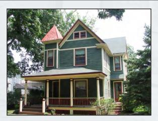
Built by H. E. Stuckslager, this house has the typical Queen Anne irregular roof and overall plan. The tower/turret with pyramidal roof at the northwest corner is also a popular detail of this style. The porch spanning the front *facade* has Doric columns with a square spindle railing. The wood bands around the house between floors add to the surface texture of the building.
