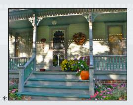
A hipped cottage with Queen Anne detail describes this charming home. Rich in texture, patterned shingles, narrow siding and the spindle-worked porch break up the exterior surface. The roof is hipped with intersecting *gables* and unusual broken *pent roof* beneath the *dormers*. A one story bay with *hipped roof* is seen at the southwest corner.
