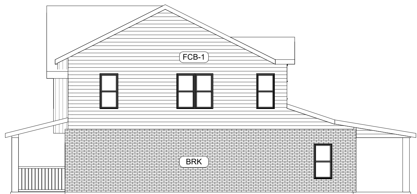
4 BLDG 2,3,4 - WEST ELEVATION SCALE: 1/8" = 1'-0" BUILDING 2 & 4 SIM.
