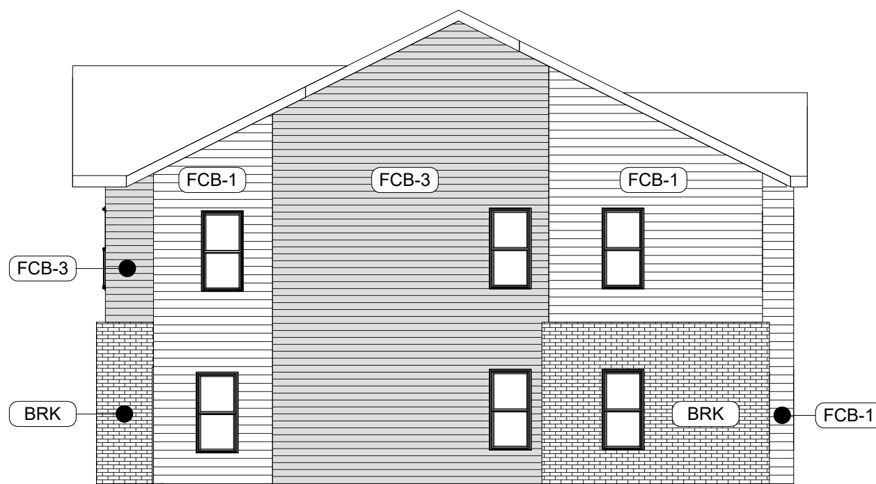
3 BLDG 1 - EAST ELEVATION SCALE: 1/8" = 1'-0"
