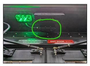
Installation of Sensors: As part of its commitment to continuous improvement, CyRide recently upgraded all low-floor buses equipped with touch bar handles on the rear doors to include a sensor that detects when passengers wave their hands. This change will make it easier for passengers to operate the back doors and reduce the potential for the doors to unexpectedly close when riders are deboarding. The Technology Coordinator and the maintenance division developed a custom circuit board to
