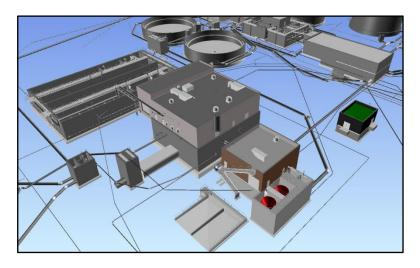
While the design of the treatment portions of the facility are complete, staff continues to work with the team from Strand Associates on the new Administration Building. Pictured is a screen capture of the 3-D design process being used to prepare the construction plans.
