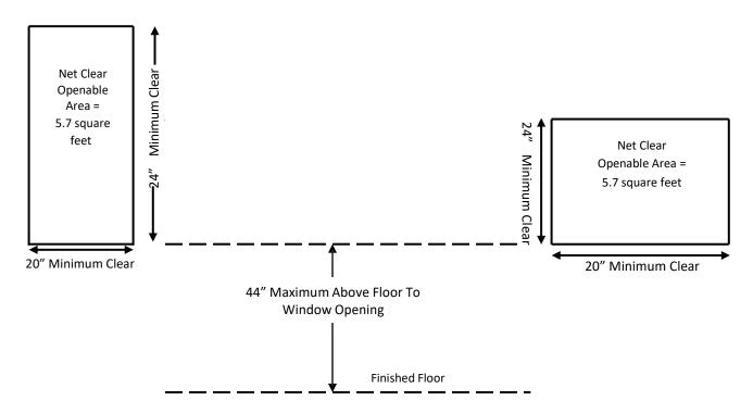
Minimum Net Clear Opening Width/Height combinations that will provide the required 5.7 square feet clear opening for Emergency Escape & Rescue Openings (inches).
